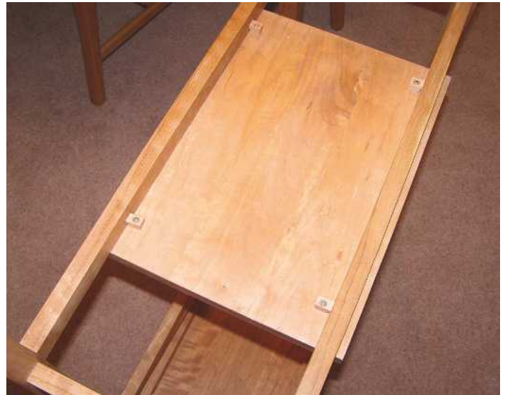
▲ Pic.16 Attach the lower shelf using four buttons
